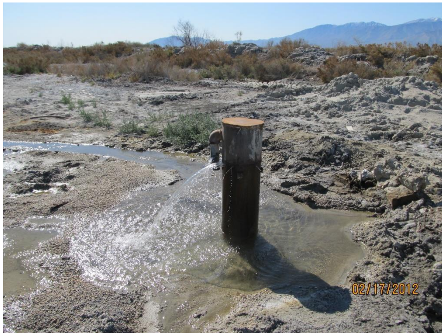
Example of an Artesian Well that would be Addressed by the Regional Well Retrofit and Abandonment Program
